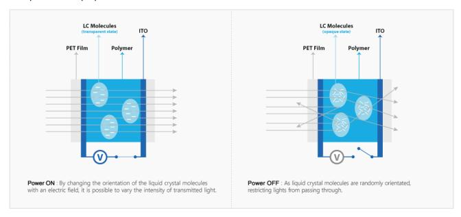
Self-adhesive PDLC smart film is manufactured with a self-adhesive cling layer on rear side, you can peel and stick to the existing glass, which provides a simple and cost effective alternative to smart glass panel.
